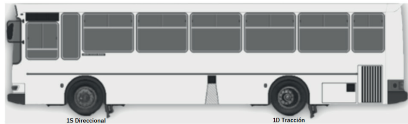
Figure 1. Axle configuration, low-floor urban bus (national jurisdiction), 2021
