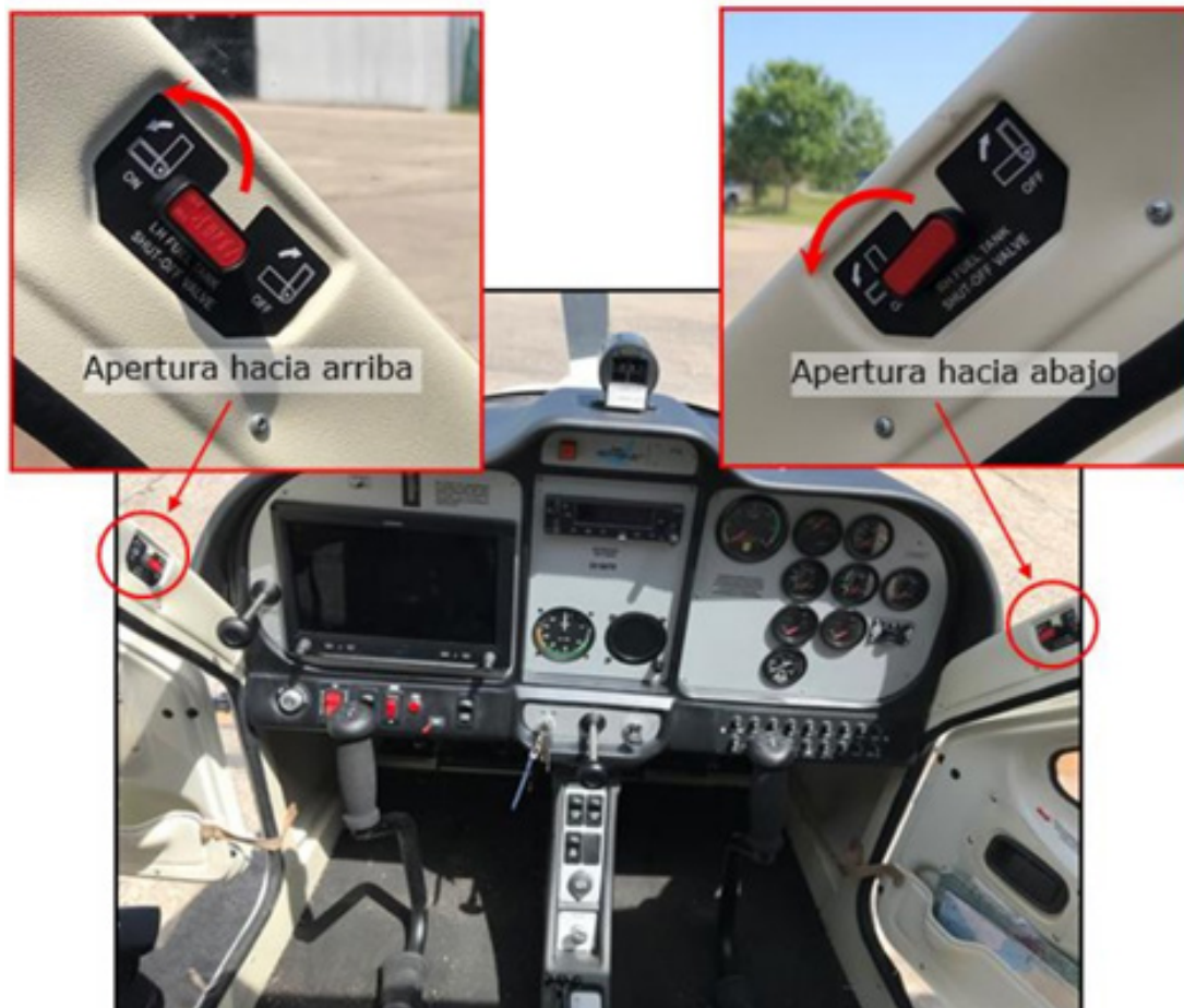
Figure 3. Fuel selector valves of an aircraft similar to the one involved in the accident
